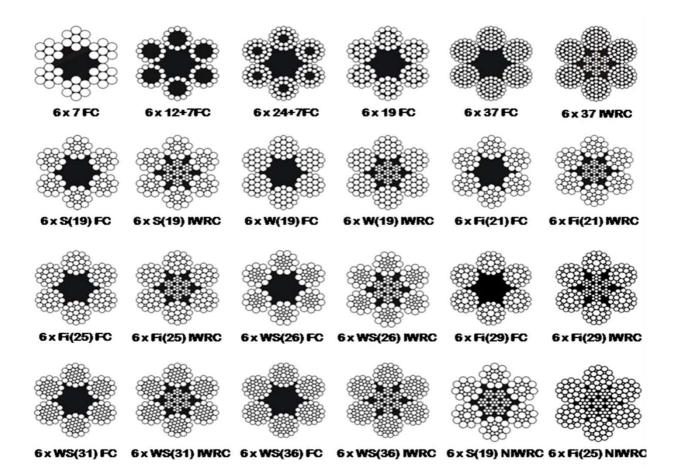
All The Above Wire Rope Available In Make Usha Martin, Orion Ropes And Other Local and Imported Make Tested Wire Rope Manufacturers.
