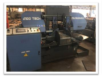
2. Full Automatic Bandsaw Machine- Dia 100-725mm
