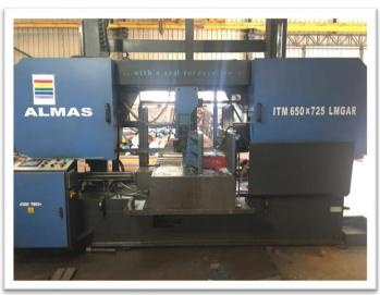
4. Full Automatic Bandsaw Machine- Diameter 70-500mm
