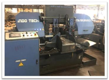
5. Full Automatic Bandsaw Machine- Diameter 100-300mm
