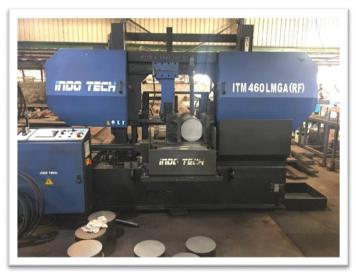
6. Full Automatic Bandsaw Machine- Diameter 100-300mm
