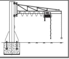
A jib crane is a type of overhead crane that does not have a runway system; instead, it attaches to a wall and extends its boom over the coverage area. These overhead cranes can also be freestanding, which means each structure has its own support column. This crane swings from 180° to 360° in a circular motion. A jib crane can lift loads of up to several tons despite its small footprint.
