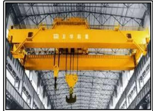
Bridge cranes are one of the most popular type of overhead crane in the market. A bridge crane have two overhead runway beams, which are connected to the building's support system. This crane is available in Single and Double girder Configurations. A Single & Double girder bridge crane has same strength. On the other hand, Single Girder are design for low capacity, Double girder crane are design for Higher capacity and can lift a load higher than a single girder crane.
